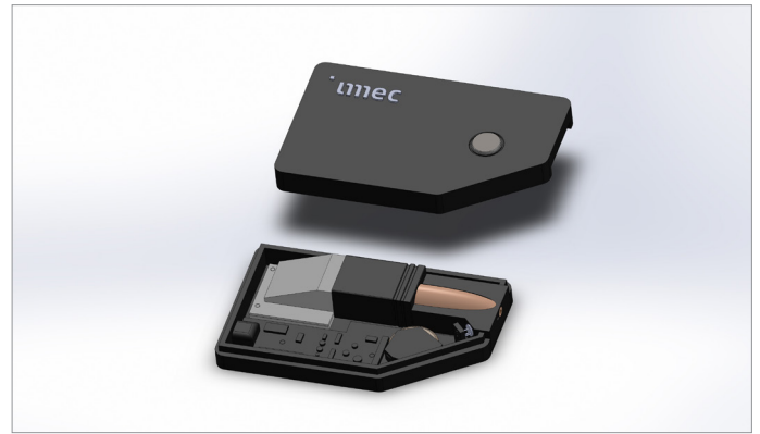
Demonstrator device for handheld high-end Raman spectroscopy.
